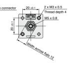
**Digital Pressure Switch ZSE30A Assembly**
