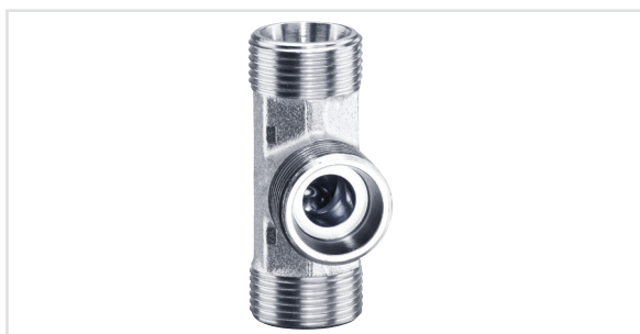
WV - Alternating valve: These valves permit the passage of flow from either inlet 1 or 2 to the outlet port whilst shutting off the inlet port not in use. The shutting off, of an inlet is achieved by a floating ball bearing which moves by the pressure of the flow.
