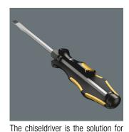
jobs that require more than just screwdriving. For fastening, chiselling and loosening seized screws or hose clamps. With an integrated impact cap that extends service live and reduces the risk of splintering. With a pound-thru hexagon blade made from highgrade material for zero-loss transfer of high forces when struck with a hammer. The tough viscous tempered material prevents the blade from splintering or breaking. More TORQUE can be transferred by attaching an open-jawed or ring
