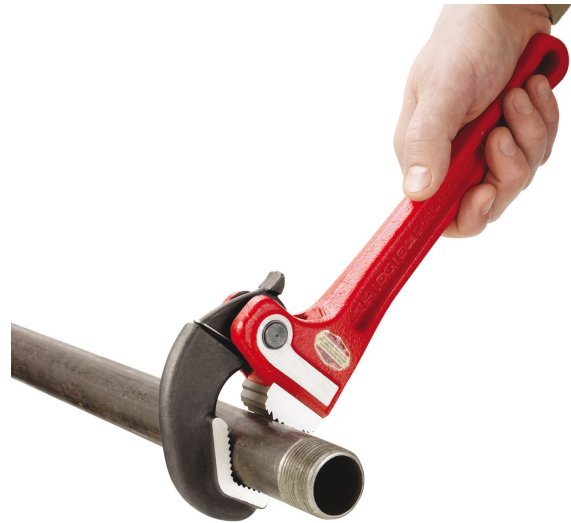
Figure 5 – Using a RapidGrip Wrench
