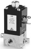
These solenoid valves are equipped with a manual override and are available with G1/8 inlet ports and with G1/8 outlets or with a diameter 4 cartridge. The body is supplied complete with screws and O-ring.
