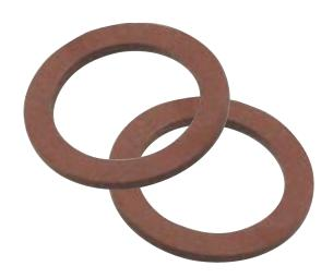
Engex sealing washers maintain the Ingress Protection (IP) rating between the equipment and cable gland. It may be necessary to fit an entry thread sealing washer at the gland entry interface. The need for a sealing washer will very much depend on the IP rating and code of protection of the equipment and the type of entry holes available within that equipment.
