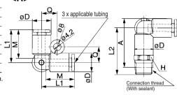
\* Reference dimensions after R thread installation.
