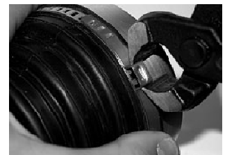
Fit clip over application. Engage interlocking hooks in tightest available position. Firmly crimp the ear with pincers.
