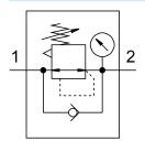
For stepless, precise adjustment of the required operating pressure
