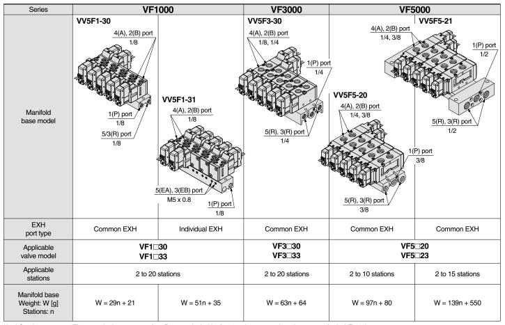
Note) Supply pressure to 1(P) ports and exhaust pressure from R ports on both sides for 10 stations or more (5 stations or more for the VF5000).
