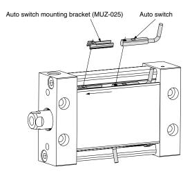
3. Confirm where the mounting position is, and tighten the auto switch mounting screw using a flat head screwdriver to fix the auto switch.
