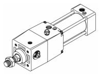
2) Remove the tie-rods, head cover and cylinder tube.
