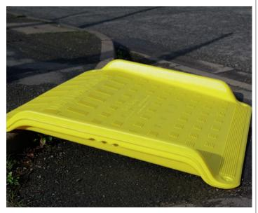
The **TRAFFIC-LINE** Kerb Ramp is manufactured in High Density Polyethylene (HDPE) for strength and durability. It can accommodate kerb heights from 75mm to 125mm and can be fixed permanently if desired via four fixing holes moulded in. The surface is embossed with an anti-trip pattern making it safe in use.
