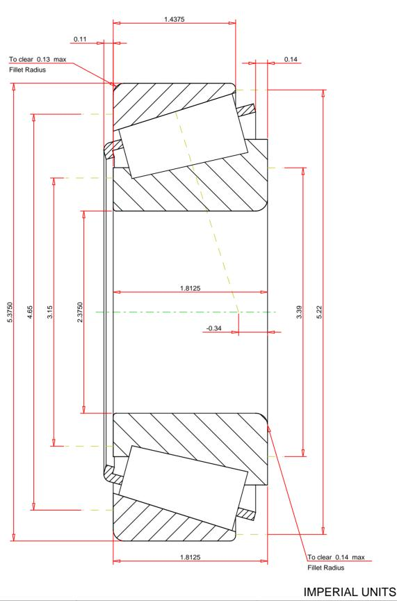
H715332 - H715311 Tapered Roller Bearings - TS (Tapered Single) Imperial
