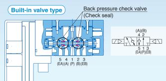
Retrofit or pre-installed type If the product is affected by back pressure after installation, the back pressure check valve assembly can be added.
