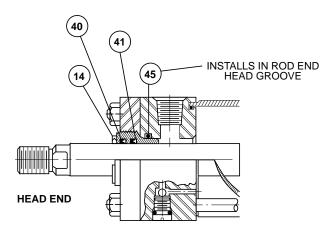
When replacing a gland on a rod which is threaded to the full diameter or so shaped that it could damage the seals, a slight rotary motion of the gland will help prevent damage. In addition, because full-diameter threads are usually supplied with the crest of the threads slightly truncated, a piece of shim stock or other thin, tough material can be wrapped around the threads to help protect the gland seals when they are being passed over the threads.
