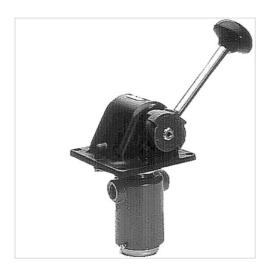
Туре Poppet valve Working pressure min./max. See table below Adjustment range min./max. See table below -25 ... 70 °C Ambient temperature min./max. Medium temperature min./max. -25 ... 70 °C Medium Compressed air Nominal flow Qn 900 l/min Hysteresis 0.15 bar Weight 1.2 kg
