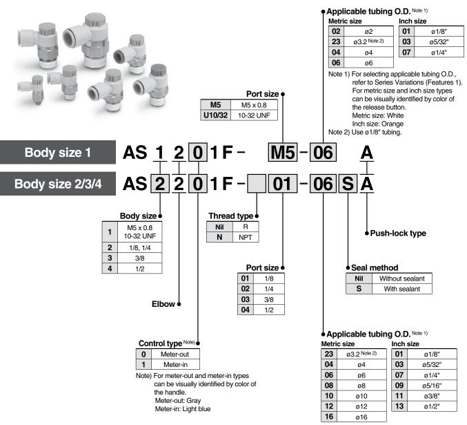
Note 1) For selecting applicable tubing O.D., refer to Series Variations (Features 1). Note 2) Use Ø1/8" tubing.
