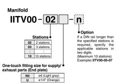
Note) A DIN rail with the length specified by the number of stations is attached to the manifold. For dimensions of the DIN rail, refer to the external dimensions.
