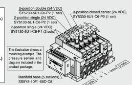
For the valve arrangement, the valve closest to the D side is considered the 1st station.
