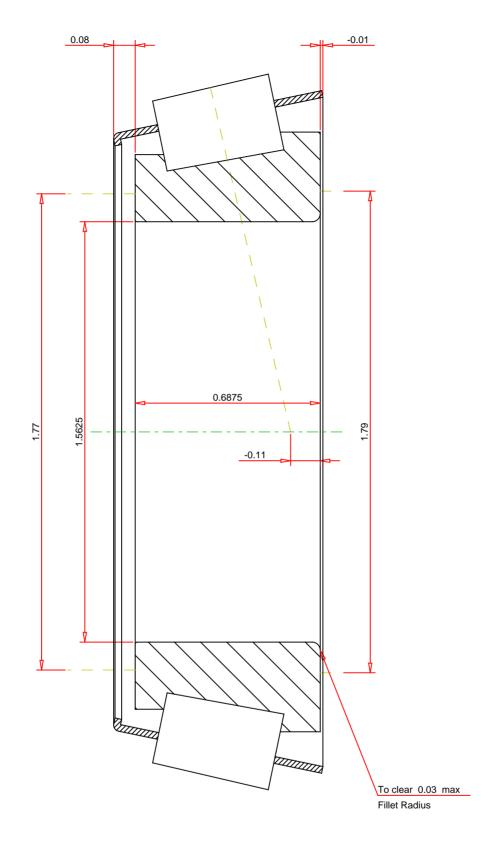
**IMPERIAL UNITS** Number of Rollers Per Row 18587 Tapered Roller Bearings - Single Cones - Imperial THE TIMKEN COMPANY K Factor Dynamic Radial Rating - C90 2960 NORTH CANTON, OHIO USA Dynamic Thrust Rating - Ca90 1770 Dynamic Radial Rating - C1 11400
