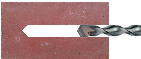
Drill correct diameter hole to correct depth
