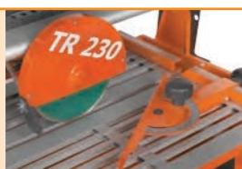
Cutting guide with angular setting
