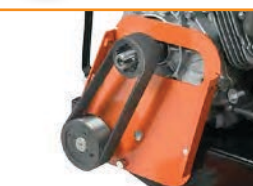
Pulleys with removable hub and Poly V belts
