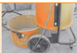
The CV324 has a removable dust bin
