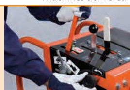
Manual or hydraulic raise and lower of the blade
