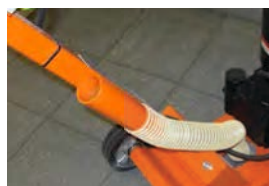
Hose connector to fit dust collector
