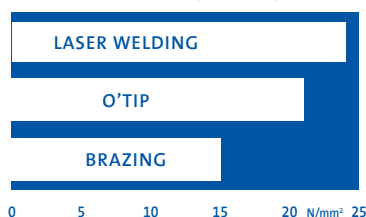
SEGMENT TORQUE RESISTANCE TO BREAKAGE (IN N/MM 2 )
