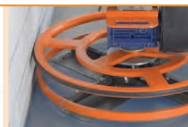
Distance to wall : 10mm
