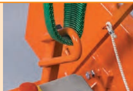
Integrated lifting hook
