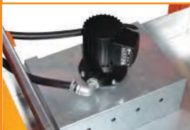
Electric water pump (Jumbo 651 6.75.3)
