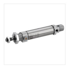
Standards ISO 6432 Internal thread Compressed air connection Working pressure min./max. 2 ... 10 bar Ambient temperature min./max. -25 ... 80 °C -25 ... 80 °C Medium temperature min./max. Compressed air Medium 50 µm Max. particle size Oil content of compressed air 0 ... 5 mg/m<sup>3</sup> 6.3 bar Pressure for determining piston forces
