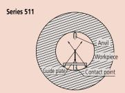
The 511 series provides a guide plate to align the setting ring diameter with the measurement axis of the bore gage.
