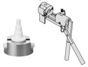
2. Tighten the nut to the end surface of the body. As a guide, refer to the proper tightening torques shown below.
