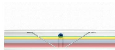
Internal fitting Fire Safety Clips
