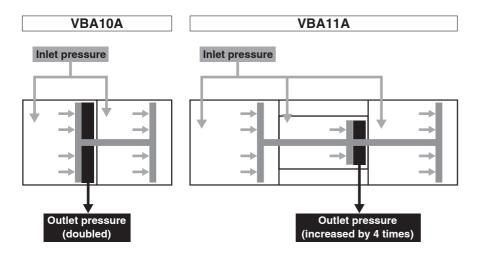
The VBA10A has two pistons and four chambers.
