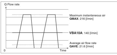
Booster regulator selection and air tank necessity confirmation results
