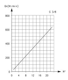
Flow Qn (Nl/min.) from  $2 \rightarrow 1$  with controller OPEN: 530 Flow Qn (Nl/min.) from  $2 \rightarrow 1$  with controller CLOSED: 160
