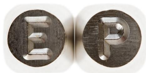
Reverse impression punches have a positive readable face to produce a negative indent - for use in forging or moulding applications, to produce a positive or readable inscription on a moulded or cast component
