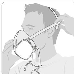
1. Place the respirator over the mouth and nose and fit the head straps as shown in the illustration.
