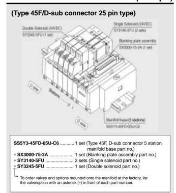
Since double solenoid 3 position valves (dual body type) require 2 manifold stations, be sure to specify the appropriate number of stations with the manifold part number. (Manifold Specification Sheet on pages 205 to 218)
