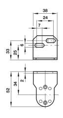
Use 1/8" (3 mm) screws to mount bracket to wall.
