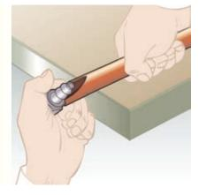
2. Grip hose and give a sharp down-ward tug to disengage from fitting.
