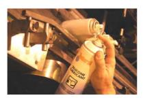
**SILICONE LUBRICANT** is a general purpose, medium duty silicone lubricant, which exhibits excellent anti-stick and slip properties.
