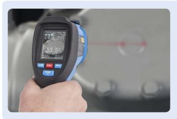
When used in non-contact mode, the thermometer senses the thermal energy radiated from an object with an infrared detector. When pointed at an object, the infrared detector collects energy, producing a signal that the microprocessor translates as a reading on the backlit display. As the trigger is squeezed, the object temperature is continuously measured by the infrared detector. This allows for fast and accurate realtime readings.
