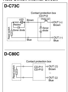
Note 1) Operating load is an induction load. Note 2) Wiring to the load is 5 m or longer. Use the contact protection box in any of the above listed situations. The contact point life may decrease. (Refer to page 1273 for contact protection box.)
