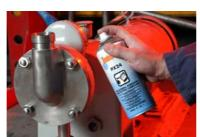
**PX24** is the complete maintenance treatment for protection against corrosion, water displacement, lubrication and light surface rust removal. One simple application – by spray, swab or dip –
