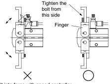
Bolt interferes with speed controller
