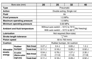
\* Operate the cylinder with in the allowable kinetic energy.
