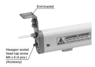
Note) The number of center brackets required, as listed below, depends on the bar length. Two end brackets are always required regardless of the bar length.
