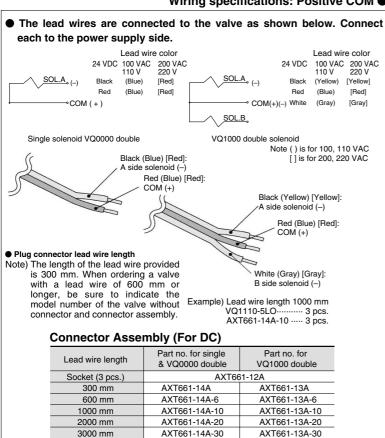
Note) 100/110 VAC for single: AXT661-31A-□; for double: AXT661-32A-□ 200/220 VAC for single: AXT661-34A-□; for double: AXT661-35A-□
