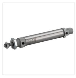
ISO 6432 Standards Compressed air connection Internal thread Working pressure min./max. 1 ... 10 bar -10 ... 120 °C Ambient temperature min./max. Medium temperature min./max. -10 ... 120 °C Medium Compressed air Max. particle size 50 µm 0 ... 5 mg/m<sup>3</sup> Oil content of compressed air Pressure for determining piston forces 6.3 bar
