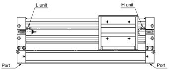
Stroke adjusting unit Example of LH attachment
