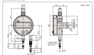
Note 1: Dimensions of the inch (ANSI/ AGD Type) dial indicator partly differ from those of the metric (ISO/JIS Type) indicator.
