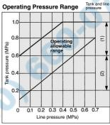
Note 1) Tank pressure is removed when line pressure is stopped.
