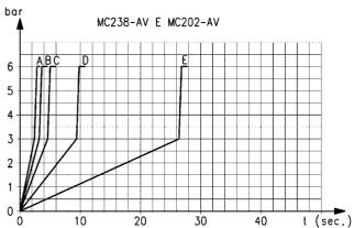
Pressurisation times as to the n° of turns of the regulation screw, with downstream volume of 5 litres. A = 5 turns - B = 4 turns - C = 3 turns - D = 2 turns - E = 1 turn. "K" = n° of turns of the regulation screw required to obtain the required pressurisation time with an inlet pressure of 6 bar. Variations of the inlet pressure can cause deviations of the pressure time by  $\pm$  20%. K = tV where: V = volume of the downstream system in litres; t = desired pressuring time in seconds.
