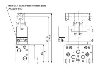
Residual pressure release valve spacer
