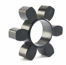
HRC Elements are manufactured from NBR/SBR rubber Operating Temperature of -40/+100°C (inclusive of rubber Element)
