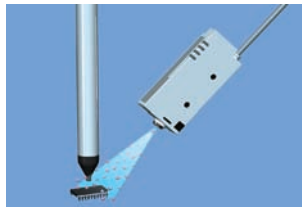
Eliminating static electricity from an IC chip
